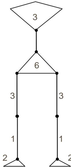
**Figure 3.** Hierarchy of the skeleton model: The pelvis is the root segment, which has six degrees of freedom (DOF) relative to the world. Numbers beside the segments represent the DOF added by that segment. The two DOFs of ankle and subtalar joint are combined in this diagram. The total number of DOF of the skeleton model is 21.
